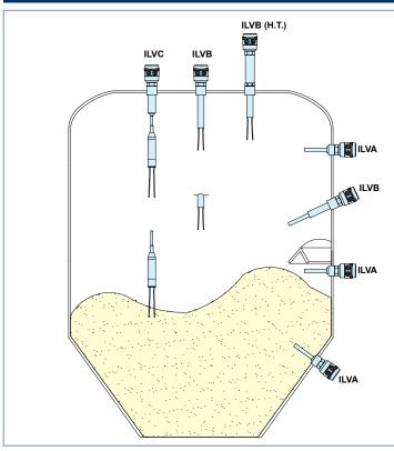
ILV Vibrating Level Indicators are fitted on the walls of a bin, silo or hopper, depending on the type of detection they have been installed for.
