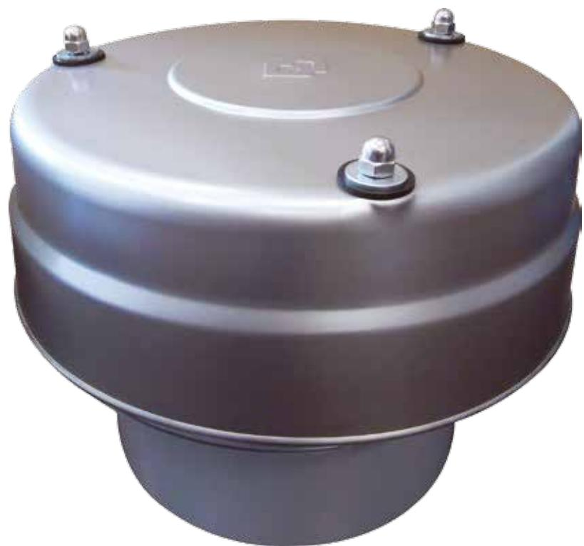
VCP Pressure Relief Valves consist of a cylindrical casing with clamped weld-on spigot, a disc shape inner steel lid for negative pressure operation held in position by a central spring rod, an outside steel ring for excess pressure kept in position by three spring rods, gaskets, and a weather protection cover.
