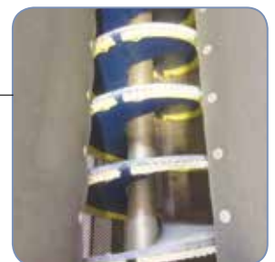
Shaftless screw with fixed centre pipe
