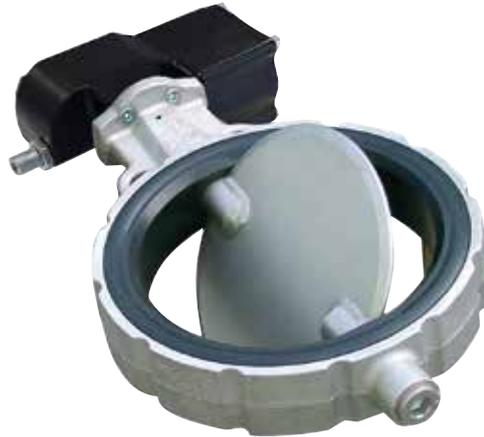
VW Butterfly Valves consist of a one-piece body made of die-cast aluminium, a mild-steel or stainless-steel valve disc including shaft journals and an elastomer gasket. An adjusting lever or a pneumatic or electric actuator can be mounted. The three WAM® actuators are perfectly interchangeable. Interchangeability of the drive shaft (standard: DIN 5482) and the universal connection option to different flange sizes result in a variety of configurations.
